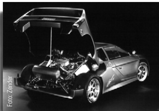
A lightweight at 55 kg, the Zender Fact 4 body shell consists of only five carbon-fibre components
