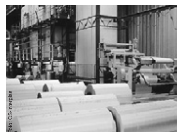
Wendewickler - Einlauf in die Finish-Anlage Rotary winder - infeed into the finishing system
