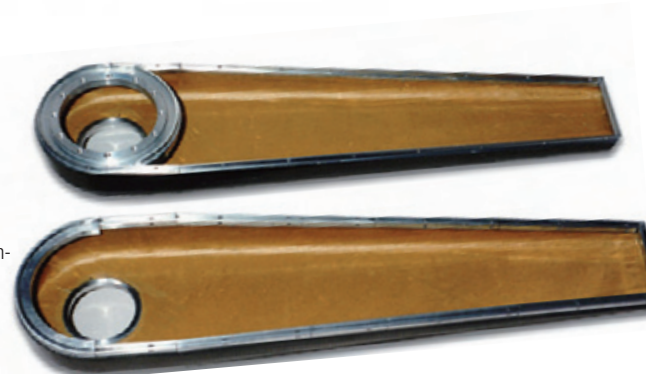
Two shells of a robot arm with glued aluminium elements and aramid fabric laminate as an internal sandwich overlay (core material aramid honeycombs)
